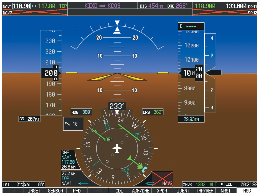
Figure 4-58 PFD1 Display after PFD2 Failure with HSDB Switch in REV Mode
